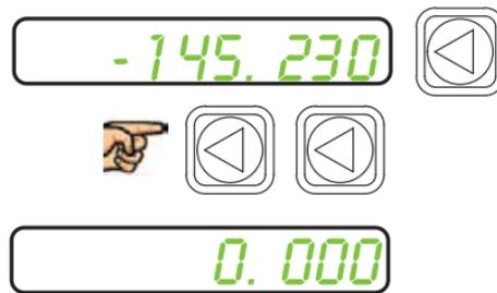
2. With the **Zero mode** selected, press the axis select key
