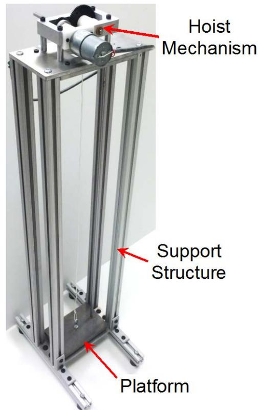
**Figure 1 – Photograph of Miniature Elevator System**
