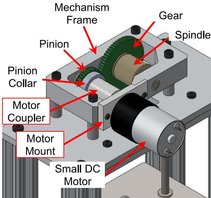
**Figure 4 – Hoist Mechanism and Drivetrain Components**
