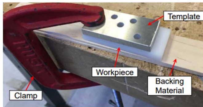
Figure 1 – Clamping Motor Mount Workpiece and Template Before Drilling
